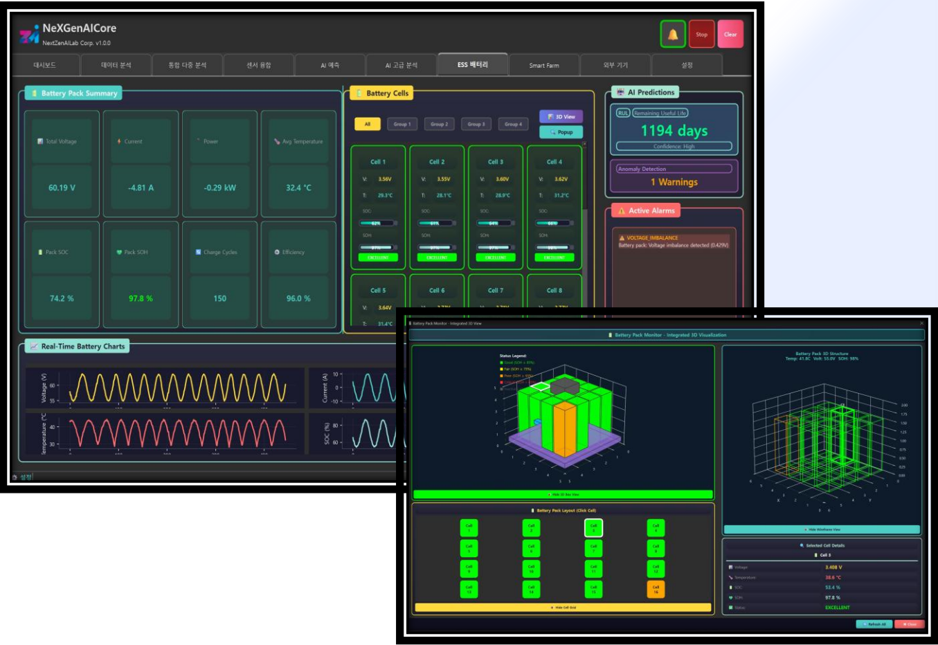
Actual Operation Screen — ESS Battery Cell-Level Monitoring — RUL Prediction, 3D Pack Digital Twin
